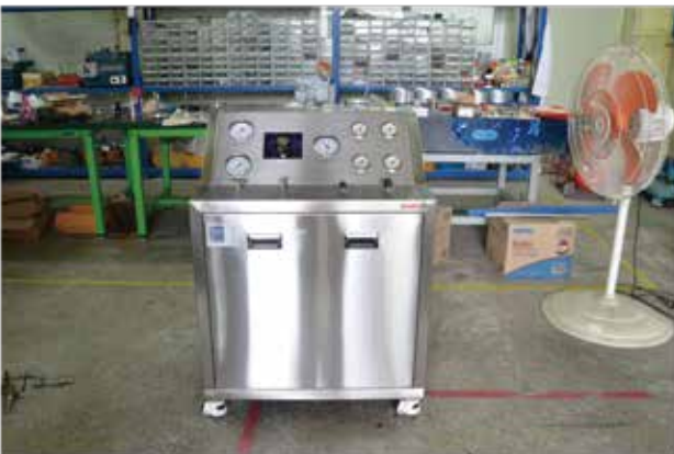
Testing module for increasing pressure and filling and spraying with propane and butane
