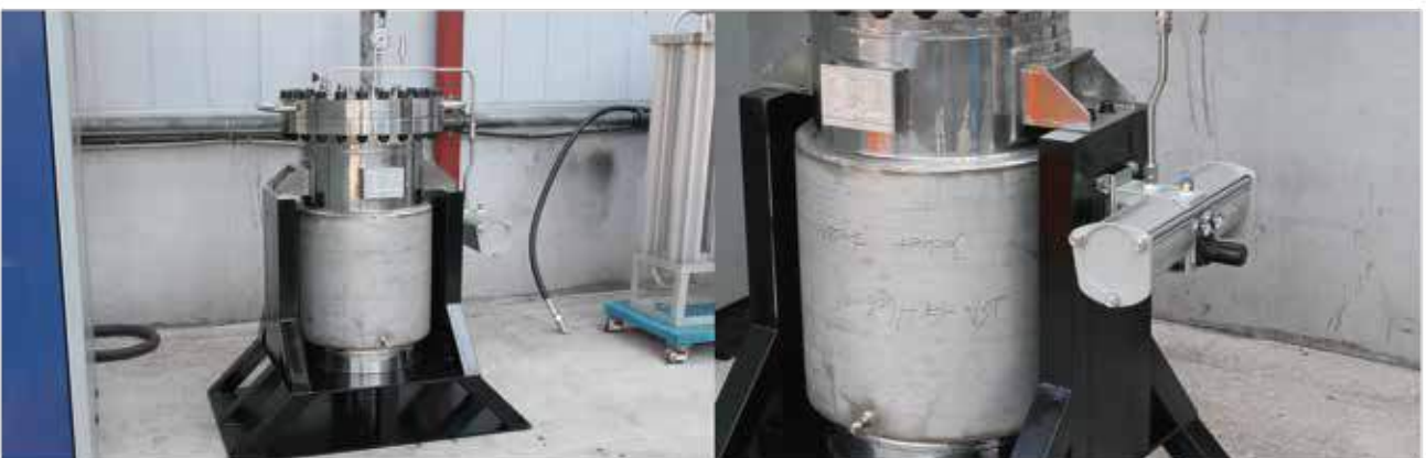
Testing module for secondary increasing pressure and filling from low-pressure compressor
