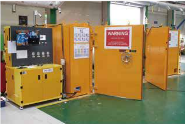
Leak testing in explosion proof purpose
