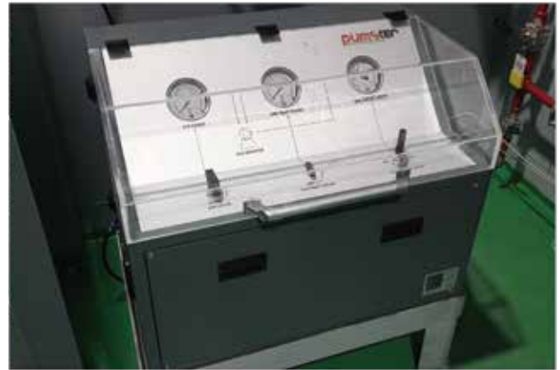
Testing module for increasing pressure hydrogen(H 2 )
